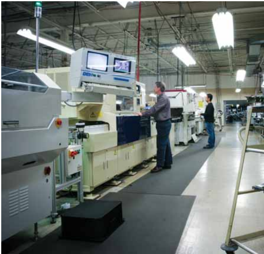
KimchuK employees assemble printed circuit boards on the surface-mount technology production line.
